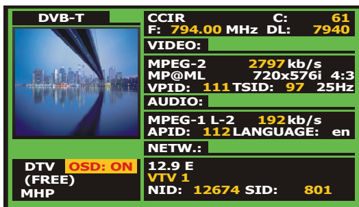
Figure 60.- Digital channel monitoring.
