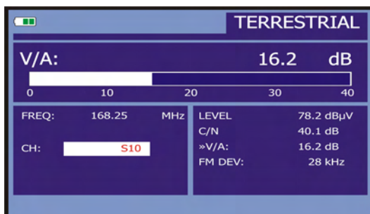
Figure 23.- Measurement of the video/audio ratio.
