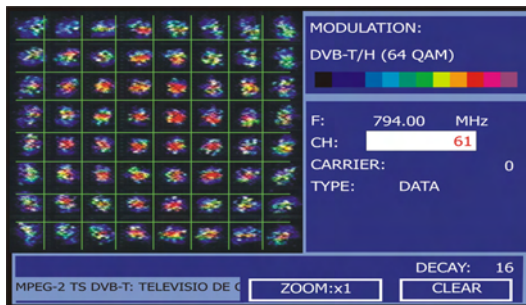
Figure 41.- Constellation Diagram. DVB-T/H (64 QAM) signal.
