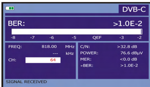
Figure 29.- DVB-C (QAM) signals BER measurement screen.
