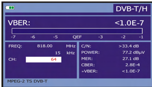
Figure 33.- DVB-T/H (COFDM) signals VBER measurement screen.
