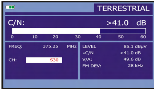
Figure 26.- Carrier-to-noise ratio measurement (C/N).
