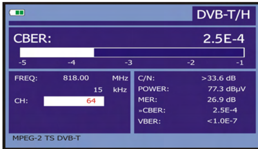
Figure 31.- DVB-T/H (COFDM) signals CBER measurement screen.
